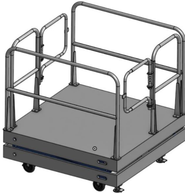
Figure II.2: Scissor Lift Model in Lowered Position
